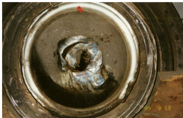
Fig. 3 Fractional leaves of the LP rotor
