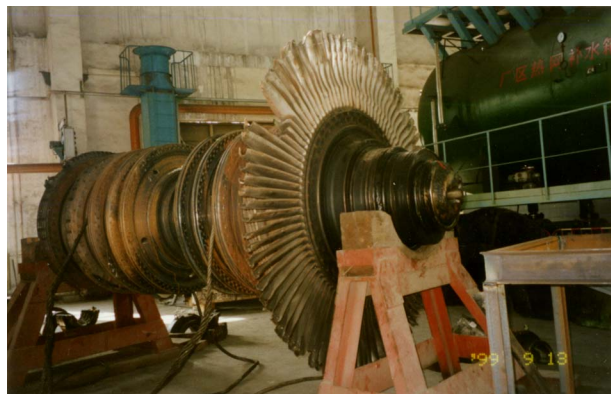
Fig. 2 Front section of the LP rotor
